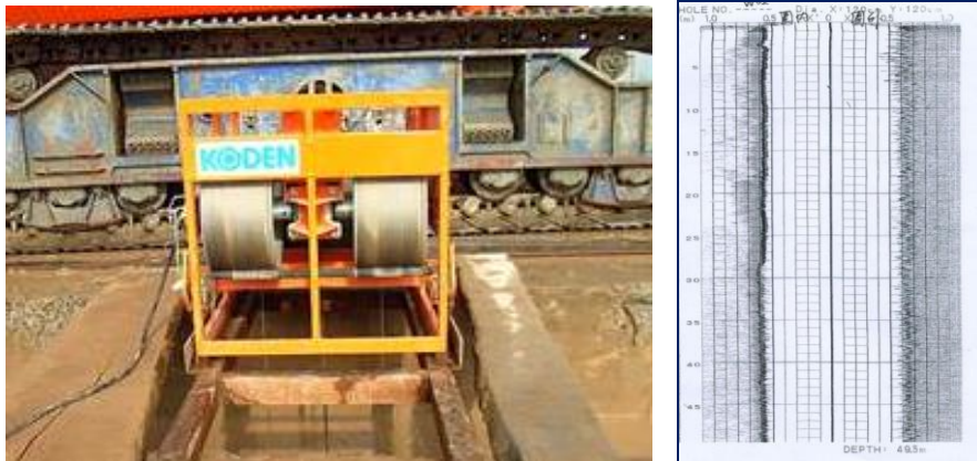
Figure 18: Kodex device and measurement log
