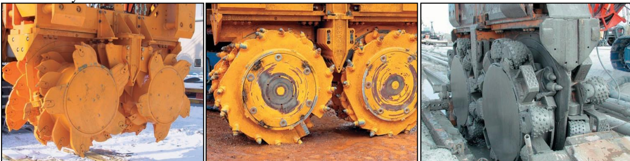
Figure 6. Standard Cutter Wheel (left), Round shank chisel cutter wheel (centre), Roller bit cutter wheel (right)
