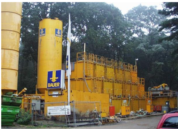
Figure 8. Bentonite storage in tanks (left); Desanding plant and bentonite storage in silos (right)
